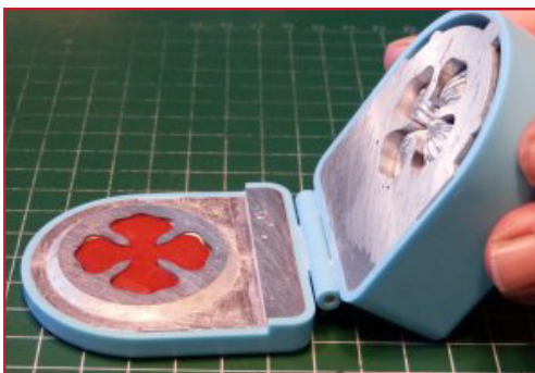
7. Emboss the clay with the emboss punch.
