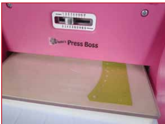
1. Cut out the Folding Die using a Die-cutting machine
